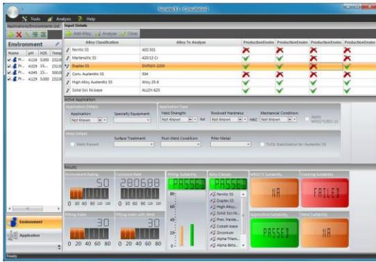
Concurrent analyses module facilitates simultaneous analysis of a select list of materials for specific environments and applications
