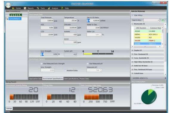
*Socrates' program interface shows a list of acceptable materials based on specified environmental conditions and application requirements*
