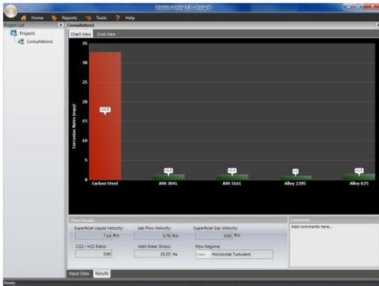
Figure 2: Predict-Amine 4.0 program output interface, showing corrosion predictions
